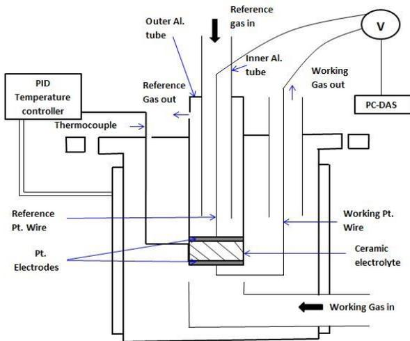
Fig. 1: Schematic of sensor testing setup
