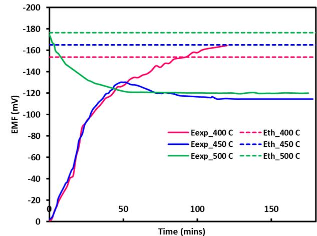
Fig. 3: Measured electrochemical potential with time at 400, 450 and 500 °C
