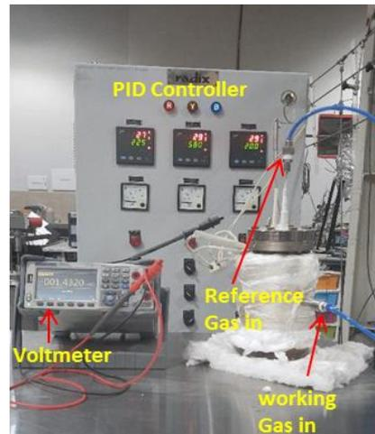
Fig. 2: Sensor testing setup
