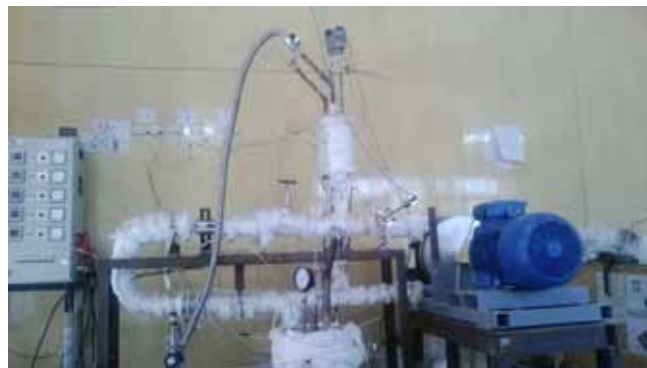
Figure A.2.4.3. Lead-Lithium loop for testing loop diagnostics
