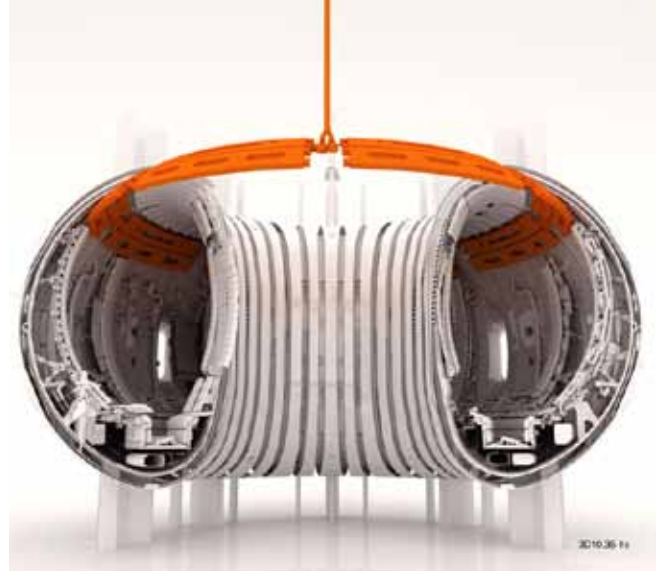
Figure A.2.6.1. A computer generated impression of the ELM control coils mounted inside of the JET vacuum vessel.
