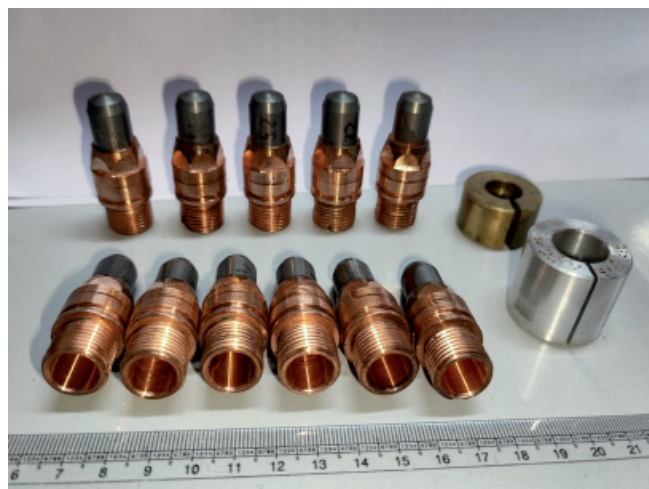
Figure A.1.12: Tungsten – Copper electrodes for plasma torch.
