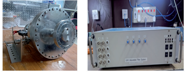
Figure A.3.32: Support structure assembly and electronics for SXR adjustable filter diagnostic.
