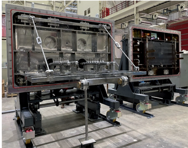
Figure A.4.5: Helium cooled and water cooled target handling systems for HHFTF.
