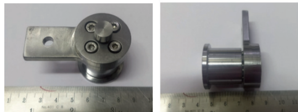
Figure A.4.6: Fixture for shear punch testing of tungsten using Gleeble 3800.
