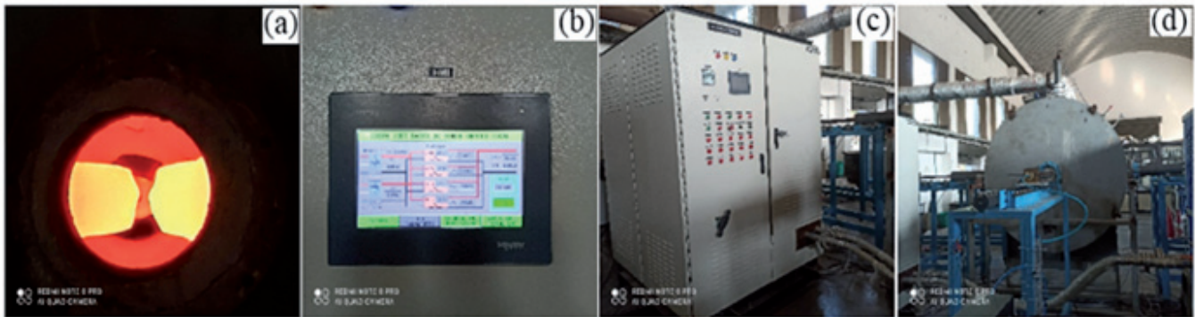
Figure A.1.10: a-Red hot electrode and chamber; b- Control Panel; c- Power supply unit; d- Plasma torch test system comprising electrodes and chamber.
