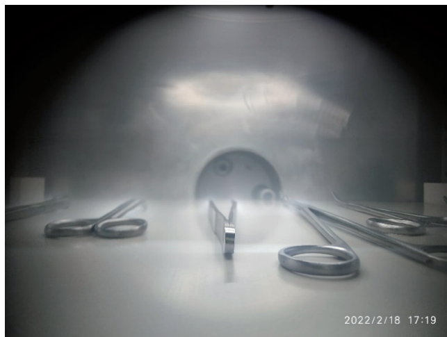
Figure A.1.11: Medical components being sterilized inside microwave plasma inside the sterilization system.
