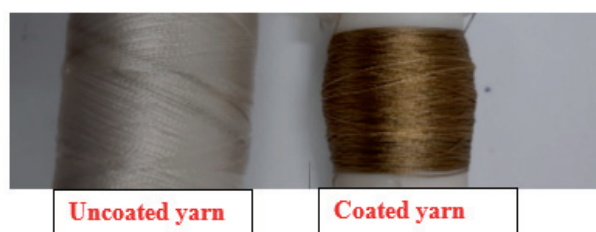
Figure A.1.2: Images of uncoated and copper oxide coated yarn.
