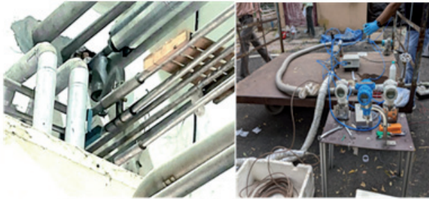
Figure A.3.8: 80 K Phase separator and Test set-up for cryo adsorber.
