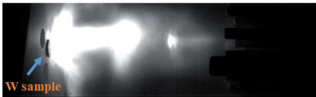
Figure A.4.9: Interaction of hydrogen plasma with W sample captured by High Speed Camera 24 mm lens, exposure 75000 frame per second.
